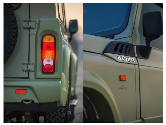
Available only with 3 doors and 4 seats, the lveco has a wheelbase of 2,452mm, making it almost identical in size to the Mercedes W461 G-Wagon SWB and Land Rover Series 2. Under the bonnet sits a 3-litre HPT 4-cylinder 16-valve turbodiesel engine, giving the Massif more than enough torque to handle even the toughest terrain, 400 Nm to be exact.
