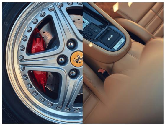
Another noticeable difference between the Barchetta and its coupé sibling is the wheels. As part of Pininfarina's distinctive design, the drop-top gained unique two-piece alloy wheels, giving the elegant bodywork a more pronounced stance on the road. Unchanged was the engine, a high-revving naturally-aspirated V12 that produced 485 bhp at 7,000rpm – creating a true orchestral exhaust note along the way.
