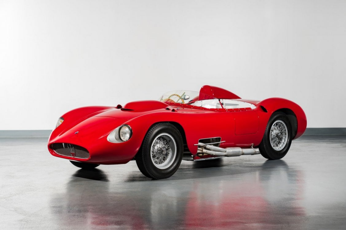
The fire-breathing 450S marked Maserati's racing swansong of the 1950s. Developed by engineer Guido Taddeucci, its chassis and gearbox had to be designed to cope with the 400 horsepower of the marque's 4.5 litre V8. One of the first cars built clocked a remarkable 181 mph with Prince Jean Behra at the wheel.
