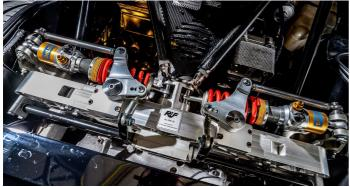
Made from billet aluminium and developed in partnership with Canadian race chassis specialist Multimatic, it's what RUF refers to as a 'birdcage' – and it lies under a flowing coat of Kevlar-carbon bodywork with barely a single straight edge to its name.
