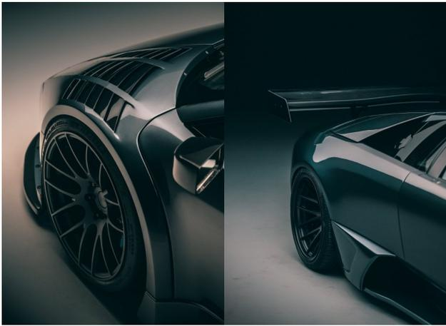
The bodywork actually features some panels from a 2008 Le Mans car; the big challenge was fitting them to a standard body. Phil adds: "There was a huge amount of fabrication that needed doing just on the parts you don't see. Then, we had to completely redesign from the door to front wing and the wings themselves. Blending the R-GT and standard LP640 sideskirts, making our own design, wider rear quarters, and so much more".
