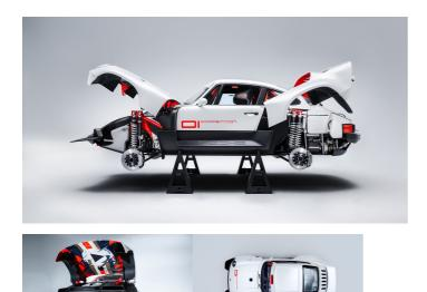
The classic twin-turbo 3.6 Porsche engine has been used with power options starting from 450bhp and 420lb ft torque. To put that power down effectively there's a 5-speed sequential dog-box enabling flat-shifting and it's manual and paddle-shift capable!
