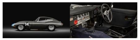
A long list of modifications was promptly made to the metallic grey coupé, including the fitment of D-type-specification wide-angle heads, Weber carburettors and uprated suspension and braking systems, to transform it from a luxurious road-going Grand Tourer to a raw and competitive racer. A strip of royal blue paint was applied to the nose, an apparent reference to a Bugatti Type 37 Protheroe had cherished in the 1940s, before the car was given its famous registration number: 'CUT 7'.
