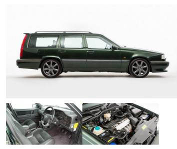
Don't be fooled by the five seats and five doors of this <u>Olive Green Volvo 850 R</u>. It may look like an ordinary family car, but with its heavy-duty manual transmission, viscous coupling limited slip differential, 2.3-litre five-cylinder engine, and turbo, this 'mum-mobile' can produce 250hp and 260lb-ft of torque. For the family who's forever fighting the clock, this estate will get you where you need to be, fast!
