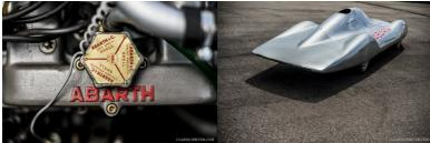
With that Coke bottle-esque shape, those distinct wheel spats, and the chopped steering wheel beneath the fighter jet-like glass canopy, the car drips poise and purpose. Its drag coefficient of 0.20 puts a BMW i8 or a Tesla Model S — two of the most aerodynamic cars you can buy today — to shame. Beneath the slippery surface resided Abarth's tiny 1,000cc 'Bialbero' four-pot, good for 100bhp and, when coupled with the four-speed gearbox, around 135mph.
