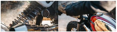
The fabulous dirt bike you're looking at is 'Super Duc', which follows the near-identical 'Dirty Duc' as the second of <u>Fuller Moto's</u> pair. It's based on a 1960s Ducati 250 Scrambler, and was built meticulously by hand from the ground up. Distinguishing features include the centre-mounted twin rear shocks, vintage Ceriani forks, and the hand-shaped headlight surround and tailpiece. Topping the bike off is an Italian-themed colour scheme in honour of the Ducati's roots.
