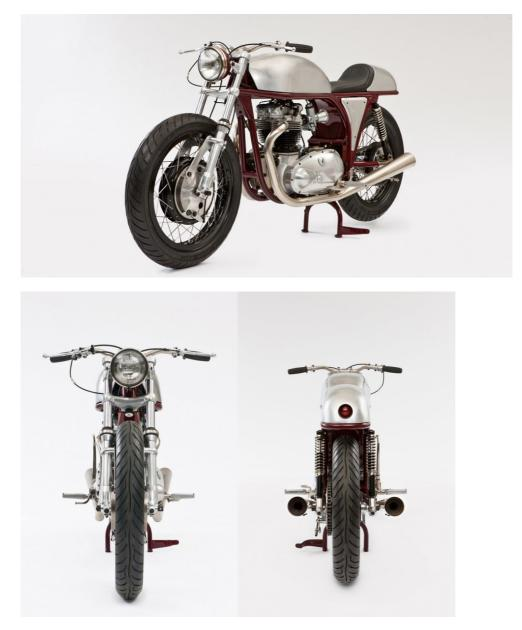
While Cleveland-based bike builder Jesse Bassett from 'The Gas Box' has used the engine from a 1959 Triumph and the featherbed frame from a Norton, a number of handmade parts such as the aluminium fuel and oil tanks have also been incorporated. To Jesse, we say kudos. We can't wait to see what's next.
