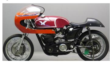
The 500cc Matchless G50 was developed in 1958 by Associated Motorcycles (AMC) at the former Matchless works in London from the highly successful 350cc AJS 7R. Approximately 180 factory G50s were made up to 1963. A race-winning package in the late Fifties, the G50 was lighter than its main competitor the Manx Norton, and as result was often more competitive on tighter, short circuits.
