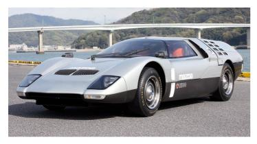
The RX500 wasn't merely an exercise for Mazda to get a slice (or, perhaps more appropriately, wedge) of the 1970s concept car action, but also a chance to showcase its revolutionary Wankel rotary powerplant. Despite being less than 500cc, the engine produced 250bhp and redlined at a screaming 15,000rpm – and for the hard of hearing, a curious set of green rear lights let those behind know when warp speed (a.k.a. full acceration) was applied.
