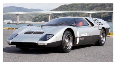
The RX500 wasn't merely an exercise for Mazda to get a slice (or, perhaps more appropriately, wedge) of the 1970s concept car action, but also a chance to showcase its revolutionary Wankel rotary powerplant. Despite being less than 500cc, the engine produced 250bhp and redlined at a screaming 15,000rpm – and for the hard of hearing, a curious set of green rear lights let those behind know when warp speed (a.k.a. full acceration) was applied.
