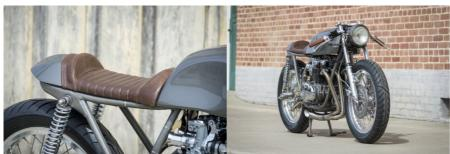
There are cosmetic features, too (though only where absolutely necessary), such as the tasteful brass highlights, a Sixties-era pressed-steel Honda headlight, and a chic, hand-built leather seat that neatly doubles as a tailpiece to house the LED taillight and battery.
