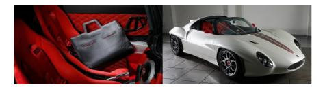
Thanks to the Kode9's aluminium chassis and numerous carbon components straight from the 3D printer, it weighs a mere 890kg. It's powered by a four-cylinder motor producing 370HP. Fully adjustable suspension and powerful brakes ensure maximum control, be it on the track or cruising the streets of Tokyo. In a tie-up with TAG Heuer (Okuyama's other love), each car is fitted with an Okuyama-designed chronograph and an exclusive leather bag.
