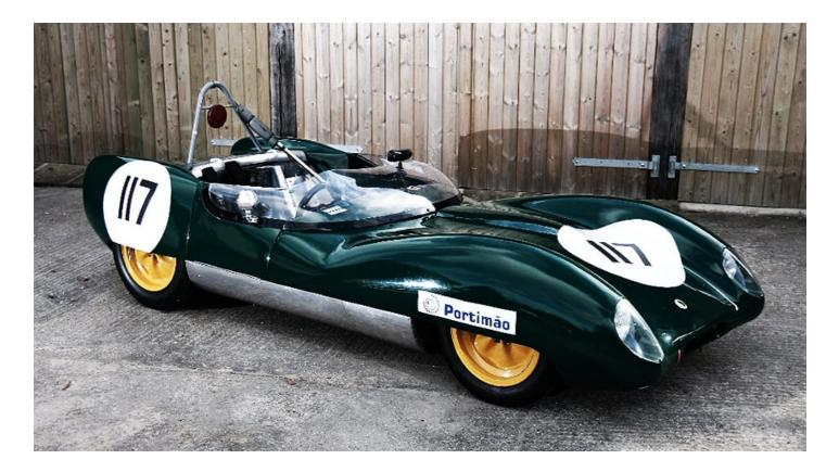
There's no denying the genius of North Londoner Colin Chapman. With the Lotus 17, his final front-engined car, he pulled out all the stops to 'add lightness' with glassfibre bodywork (a first, for customer cars) and other extensive weight-saving measures that saw the small racer tip the scales at a dry weight of just 340kg.
