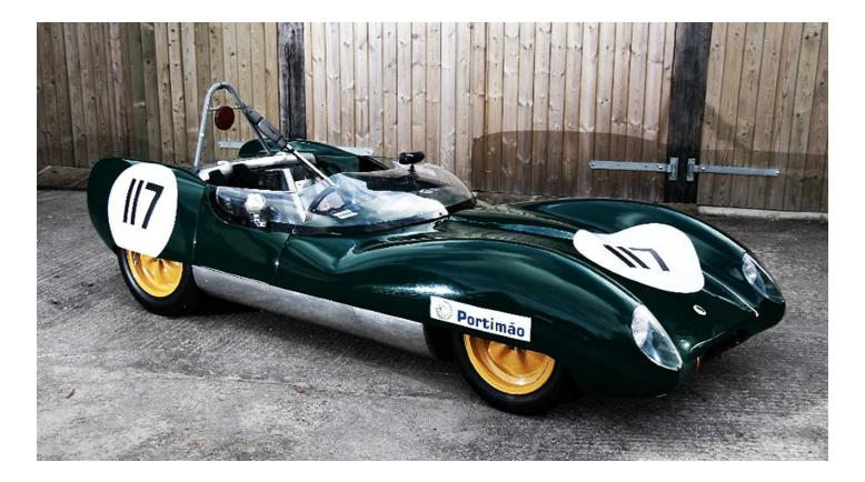
There's no denying the genius of North Londoner Colin Chapman. With the Lotus 17, his final front-engined car, he pulled out all the stops to 'add lightness' with glassfibre bodywork (a first, for customer cars) and other extensive weight-saving measures that saw the small racer tip the scales at a dry weight of just 340kg.
