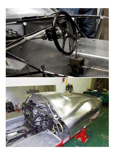
When complete, the P4 will be prepared for competition, so – as with other historic racers – some minor modifications are required to conform to modern safety regulations. For example, while the fuel tanks sit in the original area, they are now foam-filled for safety.
