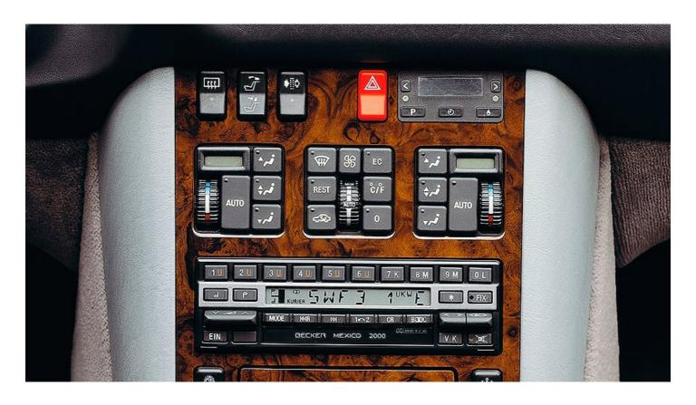
The W140 S-Class which went into production at the start of the 1990s had one of the most advanced air-conditioning systems ever seen in a car. At the time, the joys of separate temperature controls for the driver and front passenger were almost unheard-of; never mind such details as seat heating on all four seats, and the activated carbon filter that took pollutants from the air when the sensor detected them in the cabin.
