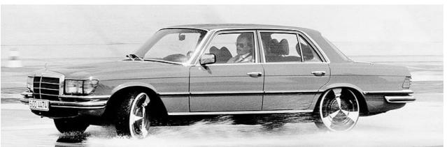
From the autumn of 1978, Mercedes-Benz offered the 450 SEL 6.9 W116 series, boasting optional anti-lock brakes that had been developed in partnership with Bosch. While ABS is today taken for granted in even the smallest and cheapest production cars, its launch in the '6.9' created a sensation.
