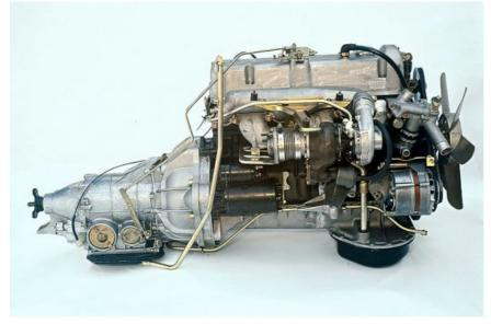
From May 1978, the W116 model range welcomed the 300 SD engine, a forerunner of today's familiar luxury diesel. The 3.0-litre five-cylinder diesel-engined version came complete with a turbocharger – Europe's first
