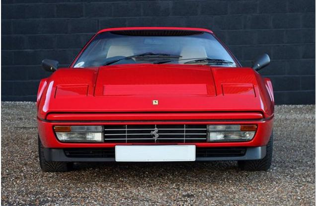
In the mid-80s, the elegant shape of the open-topped 308 GTS was further softened and rounded to become – once a 270bhp 3.2-litre engine had been fitted amidships – the 328 GTS. The curvier body not only updated the looks, it also improved the aerodynamics. Inside the new drop-top, the now outdated 1970s seats and trim and switchgear were also thoroughly refreshed.
