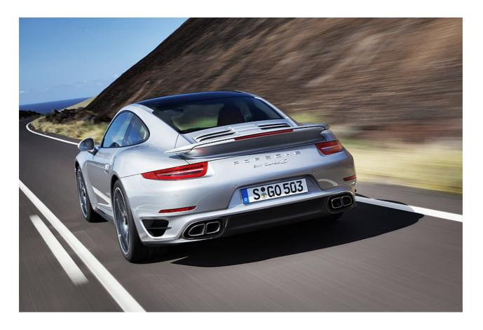
The Turbo is visually differentiated from more sedate 911s not only by its traditional signifiers such as the wider arches (the 991-gen Turbo is the widest road-going 911 ever) and the vents on the rear haunches, but also its new all-LED headlights – with camera-based beam control – and two-tone forged 20-inch wheels. The latter will have central locking hubs on the Turbo S.
