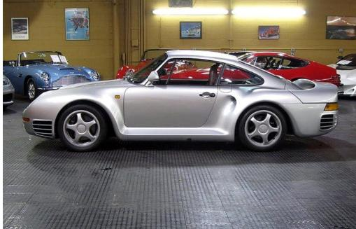
Few cars of the 1980s high-performance 'arms race' were more complex and expensive than the Porsche 959: a 4WD car created by the homologation process for racing and rallying. It was powered by a 450bhp version of the company's famous turbocharged flat six. For the first time in a production Porsche, the engine featured four-valve, water-cooled cylinder heads.
