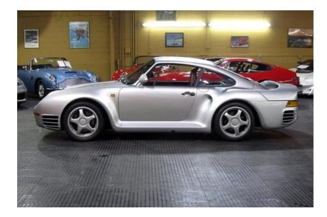
Few cars of the 1980s high-performance 'arms race' were more complex and expensive than the Porsche 959: a 4WD car created by the homologation process for racing and rallying. It was powered by a 450bhp version of the company's famous turbocharged flat six. For the first time in a production Porsche, the engine featured four-valve, water-cooled cylinder heads.
