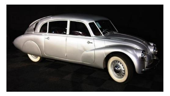
As a successor to what is commonly known as the first aerodynamically-focused production car, the Tatra T87's evermore streamlined shape made it the 'bahnstormer of its day, with near-100mph capabilities. The rear tailfin and side louvres (feeding air to the rear-mounted V8) provide the T87 with further charm – and ensure it isn't mistaken for a stretched Beetle by the uninitiated.
