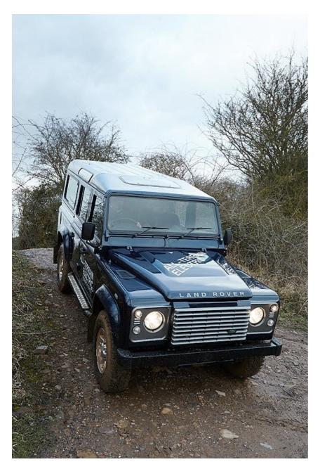
Under the bonnet, instead of a lusty diesel there sits a 410kg, 300-volt, lithium-ion battery with a capacity of 27kWh, giving a range of more than 50 miles. "In typical, low-speed, off-road use it can last for up to eight hours before recharging," says the British company. It powers a 70kW (94bhp), 330Nm electric motor that drives all four wheels via the Defender's existing four-wheel-drive system.
