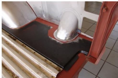
While the turbo engine is transported to a specialist for renewal, LandyPoint takes care of the axles, suspension, brakes and transmission. The chassis is also sandblasted and renovated, then remarried to the body and sealed.
