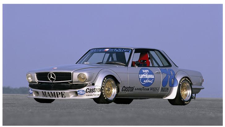
The 450 SLC had one of the biggest engines on the grid. And monstrous BBS split-rim wheels with 'cones' ducting air to the brakes. Compared with the Alpina-prepared BMWs it was a bit of a brute.
