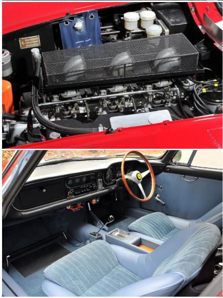
Under the bonnet, though, was a highly tuned 3,300cc V12 with high-lift cams, three bigger-than-normal Weber carburettors and a stronger crankshaft and pistons. The tubular chassis had been lightened and the Scaglietti-designed bodywork was from the thinnest-gauge aluminium possible. A big-capacity racing fuel
