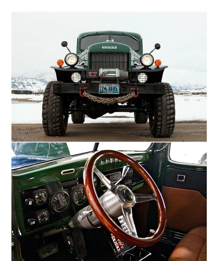
Two powerplants are available: a 426 Legacy Magnum V8 425bhp petrol, or a 3.9-litre Cummins Turbo-Diesel with 480lb ft of torque. Either a 5-speed manual or 4-speed automatic can be specified.
