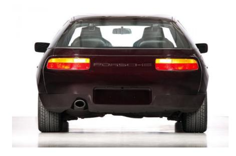
A new-at-the-time Series 4 model served as a basis, with its enlarged, now 5.0-litre V8 (tweaked to 330bhp) remaining front-mounted. The existing chassis was lengthened to give rear passengers more legroom and they were now also aided by the addition of half-sized coach doors. However, after 5,000 miles of developmental testing, the engineers decided that the chassis didn't meet the required rigidity benchmarks in elongated form, and it was swiftly consigned to storage.
