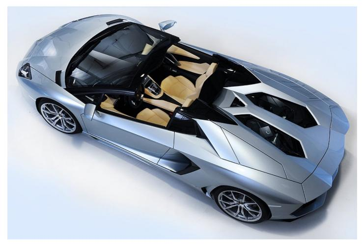
A powered rear window allows driver and passenger to govern the amount of engine noise coming into the cabin. This, in conjunction with a wind deflector that attaches to the front windshield, helps reduce wind noise and buffeting at high speeds, roof removed.
