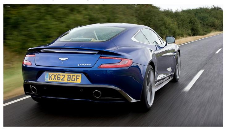
At the tail we find a spoiler flying above the main boot surface but moulded seamlessly into it, while around the body's lower edges the splitter, diffuser and lower sills parade their carbonfibre in glossy nakedness. Bumpers remain in deformable plastic.
