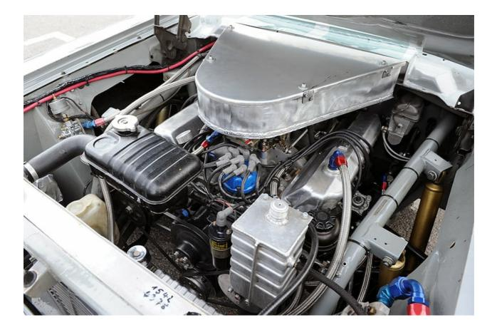
With a 427c.i. side-oiler V8 (period original, and with many features such as cross-bolted main bearing caps unique to this type of engine), it easily swallows Goodwood's rolling straights. What's surprising, though, is how well it copes with the slower corners, including the famous Goodwood chicane. And, despite fears to the contrary, with judicious restraint on the throttle it kept to the circuit's strict noise regulations, too.
