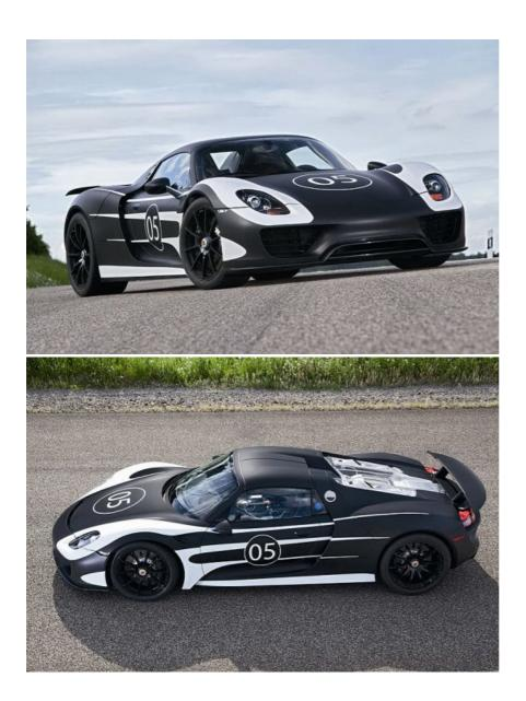
At the heart of the modern miracle is a 4.6-litre V8, mounted amidships and joined by a hybrid module on the rear axle (which also has adaptive steering) and an electric motor on the front axle. The technological showcase continues with a full carbonfibre reinforced plastic (CFRP) monocoque, fully adaptive aerodynamics, and an upward-venting 'top pipes' exhaust system.
