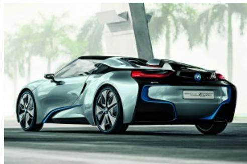
The 4.4m-long and 1.9m-wide i8 Spyder stands just 1.2m high, making it as low as a Ferrari 458 Italia. Despite the lightweight concept with extensive use of CFRP (carbonfibre reinforced plastic), the BMW comes in at a hefty 1.63 tonnes. Adding to the weight is the high-capacity battery, fitted low to keep the centre of gravity as close to the ground as possible.
