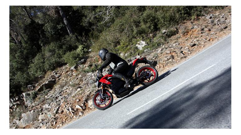
No, once under way, they really do go, corner and stop like 'proper' bikes. There's a little buzzing when the regenerative braking steps in, just to reassure you that you are getting something for nothing. In addition to their virtually silent operation, the bikes generate little heat. With this, no fuel, and belt-drive, it's all very clean and tidy.
