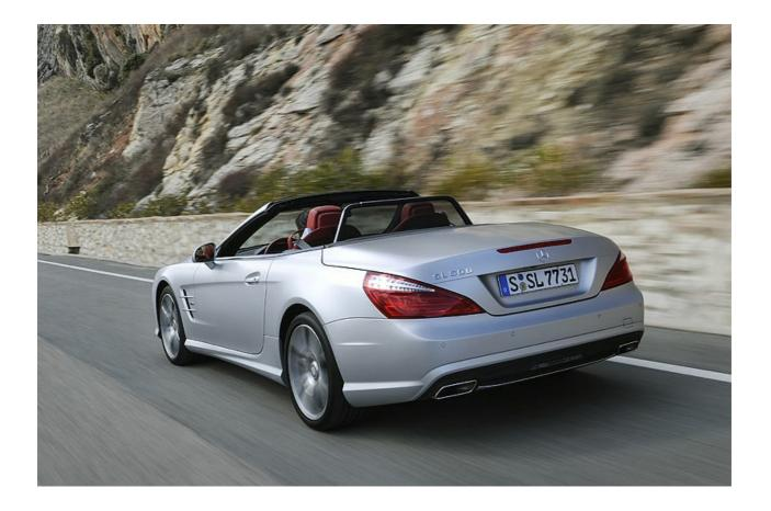
On the plus side, there is never the slightest tremor from the open-top structure, wind noise with the roof up is practically zero, and roof-down the wind rush is never so vigorous as to become wearing, especially with the electric windblocker deployed. The drag coefficient is just 0.32 with the roof down, a result even more impressive than the 0.27 roof-up figure.
