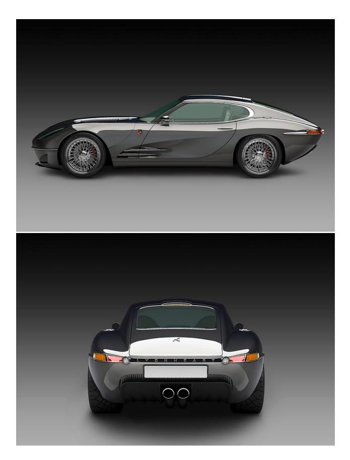
However, because the hand-built K has bodywork built entirely from carbonfibre, it has a kerb weight of 1575kg; an impressive 178kg less than the XKR-S. Lyonheart maintains this will shave up to half a second off the Jaguar's 4.2-second 0-62mph sprint.
