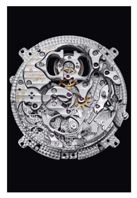
Powering the watch is a Cartier 9402 MC movement, comprising 447 parts and 47 jewels, and the tourbillon ensures the most perfect timekeeping whatever the angle of the watch. For special customers, the watch can be set with baguette-cut diamonds.
