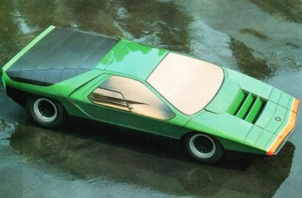
Because of its underpinnings, designer Marcelo Gandini had the opportunity to create a car that would revolutionise the automotive industry for many years afterwards. The engine being mounted amidships allowed for a pointed front end, while the ground-hugging poise inherited from the Tipo race car meant the car was under a metre tall at its highest point. Combined with the squared-off rear end, these characteristics
