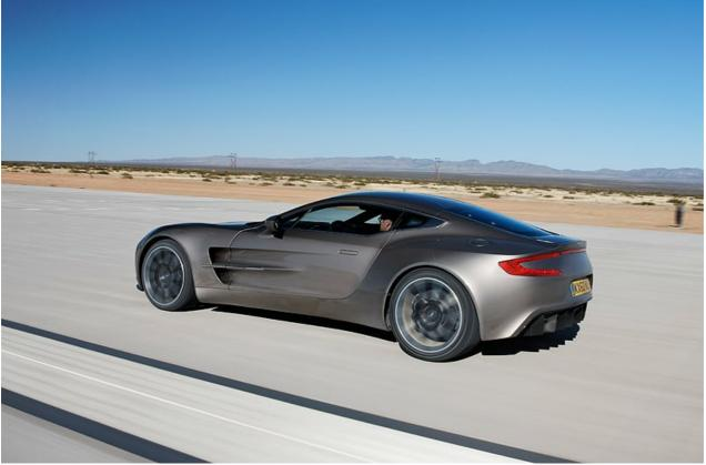
The One-77, which costs about five times the price of a space trip, is also more exclusive – with production limited to 77 cars; hence the One-77 moniker. It features a full carbonfibre monocoque with aluminum body panels and front mid-mounted 7.3-litre normally aspirated V12 engine, putting power to the rear wheels through a rear mid-mounted 6-speed automated manual gearbox.
