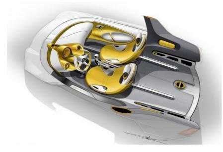
One of the concept's unique features is an electrically powered cargo tray, which slides rearwards by 280mm to aid loading.
