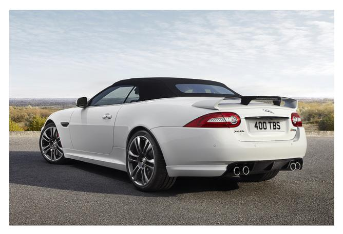
Wider wheels, forged for lightness, complete the mechanical modifications, while the body gets a new nose with slots ahead of the bonnet, a carbonfibre splitter and side ducts which channel air along flared-out sills. Carbonfibre forms the new rear wing and lower valance too, all designed for extra stability and reduced lift at high speeds.
