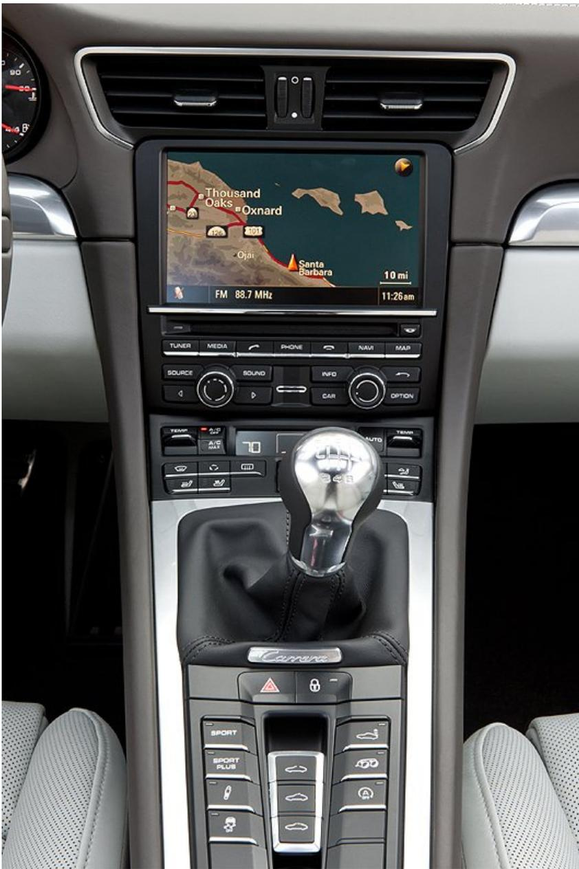
However, the seven-speed shift selects gears perfectly cleanly, and most of the time you just use it as a close-ratio six-speeder. Seventh is out to the far right and forward, upon which the lever leans at a drunken angle; an interlock prevents you from going straight there from fourth or vice-versa.
