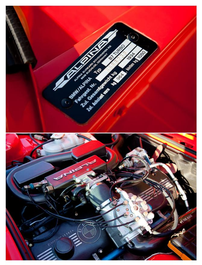
In developing the straight-six, no expense was spared. In addition to the turbocharger (a technology in its infancy in road cars then, and only just appearing on the race track), Alpina fitted all-new ignition, fuel injection and a bespoke inlet manifold.
