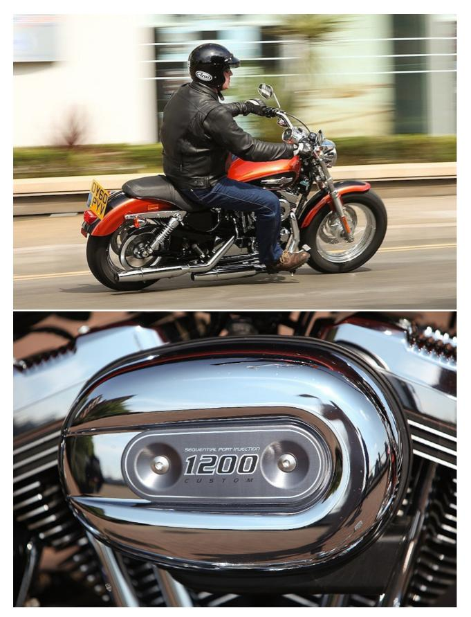
Ride quality is poor. The rear suspension is both under-sprung and a little under-damped. Hit a bump, even a small one, and chances are that the rear suspension will bottom out and, without your legs and feet beneath you to absorb some of the shock, it can be quite uncomfortable.
