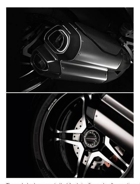
The road wheels are new to the bike, being five-spoke alloy creations of a style similar to that fitted to AMG motor cars.
