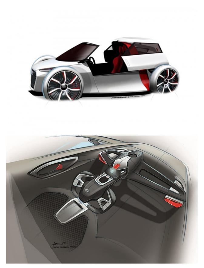
The 21in wheels run under wheel-shaped covers housing strips of LED lights that 'blink' when the vehicle is in motion.
