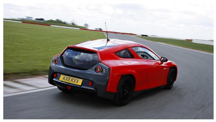
Out on the Stowe circuit section the Delta stays almost flat in the corners, brakes progressively with no detectable changeover point between electric regenerative braking and the physical, frictional variety, and feels very agile. The Ford Fiesta-sourced electric power steering self-centres poorly in this application, though, no doubt because of the lack of weight working against it, and feels oddly glutinous.
