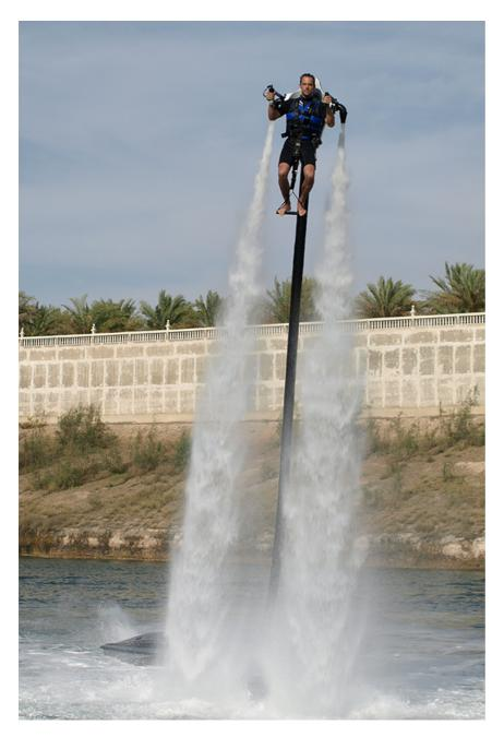
The first production versions of the German-built Jetlev were due to be delivered this month. For 129,000 euros, buyers will get a floating, carbonfibre pod containing a 250 horsepower propulsion engine that shoots a powerful water jet through a 30-foot hosepipe and into a 30lb pack strapped to the user's back with a quick release harness. The water emerges at massive pressure from two articulated nozzles built into the pack, giving more than 500lb of thrust for movement and propulsion.
