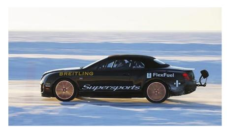
There were only minimal modifications to the car to prepare for the record-breaking drive: a fully welded, heavy-duty safety rollcage, along with Pirelli winter tyres and a rear bumper-mounted parachute, with front and rear spoilers for high-speed stability.
