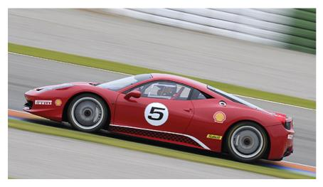
The suspension features stiffer springs, single-rate alloy dampers, centre-nut 19in forged rims, larger dimension **Pirelli** slicks and a ride height lowered by 50mm all round. The car is equipped with **Brembo CCM2** brakes, as per the **599XX**, **Ferrari's** extreme experimental laboratory car.
